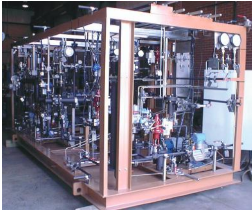
Engineered Module Tritium Removal Facility LPCE Skid
