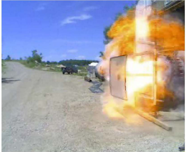
Activation of Explosion Vent by Corn Starch deflagration in 100 cubic meter test vessel
