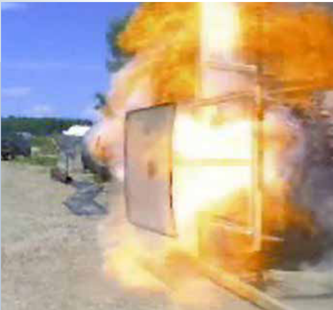
Dynamic testing of a VSB building vent
